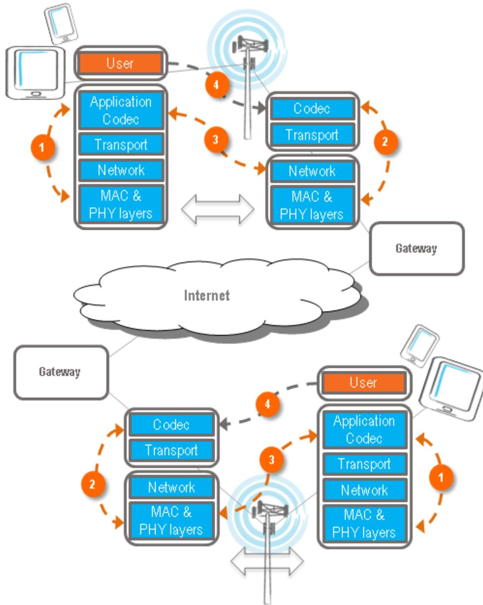
Figure 1: Different classes of cross-layer approaches to enhance video performance over wireless networks including: (Classes 1 & 2) joint optimization of the video application with the MAC/PHY at the subscriber terminal and basestation respectively, (Class 3) joint optimization of the video application in the UE and the MAC/PHY in the wireless network, and (Class 4) optimizing the video application in the network based on the state of the user.
