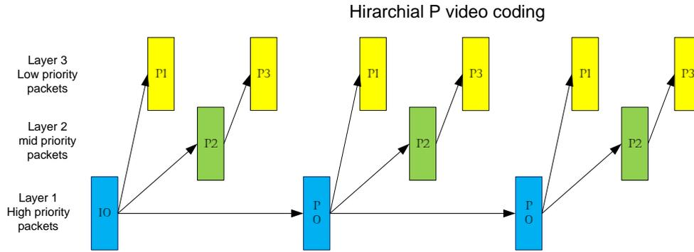
Figure 1 : Hierarchical P video coding frame priority guidelines.
