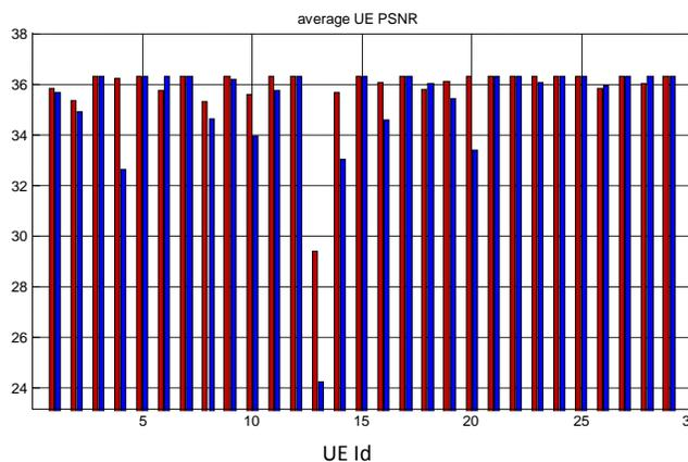
Figure 3: Objective Video Quality Measure (PSNR) per user [dB] (Fixed HARQ – Blue; Adaptive HARQ – Red)
